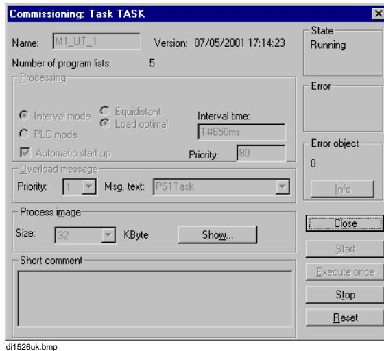
If configured for **autostart**, the task starts automatically when the resource is started. All lower-level program lists and programs start along with the task as long as the program list parameter has been set **ON**.
