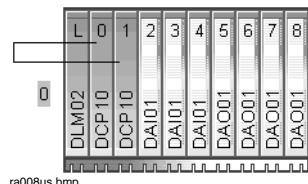
It is also possible to mount one redundant DCP10 module in the basic unit, and the second one in the extension rack.
