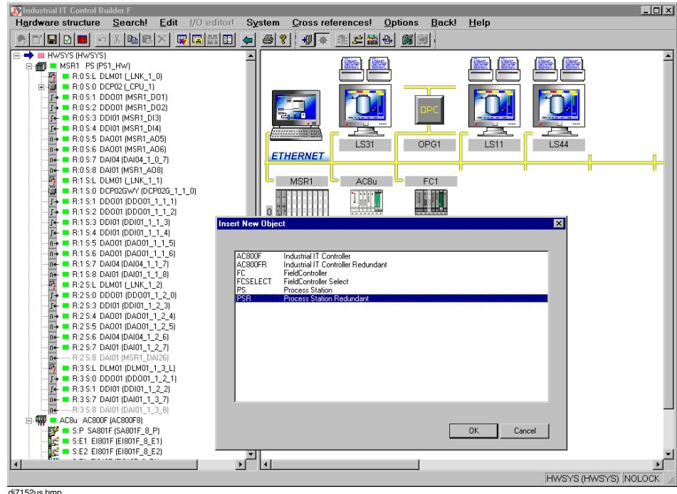
A redundant process station always features 2 CPU modules. Redundancy link is automatic when inserting a second CPU module.
